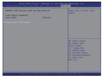
5. When the screen as shown above displays, using the arrow key, select the item "Proceed with flash update" and press the <Enter> key. You will see the progress of BIOS recovery as shown in the screen below.
