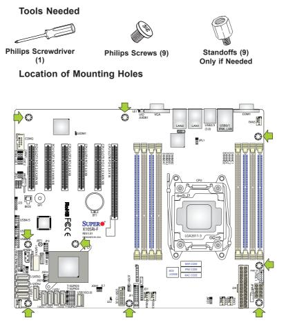
**Caution:** 1) To avoid damaging the motherboard and its components, please do not use a force greater than 8 lb/inch on each mounting screw during motherboard installation. 2) Some components are very close to the mounting holes. Please take precautionary measures to avoid damaging these components when installing the motherboard to the chassis.
