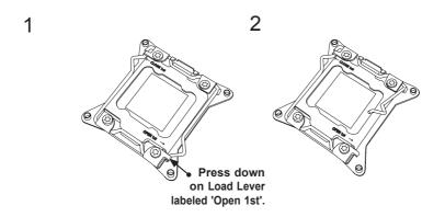
2. Press the second load lever labeled 'Close 1st' to release the load plate that covers the CPU socket from its locking position.
