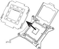
5. Using your thumb and index finger, hold the CPU on its edges. Align the CPU keys, which are semi-circle cutouts, against the socket keys.
