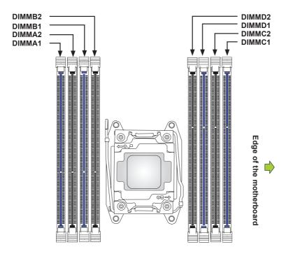
The X10SRi-F supports up to 256GB of RDIMM and 512GB of LRDIMM DDR4 2400 MHz (max.) in eight memory slots. Populating these DIMM slots with a pair of memory modules of the same type and size will result in interleaved memory, which will improve memory performance. Please refer to the table on the next page:
