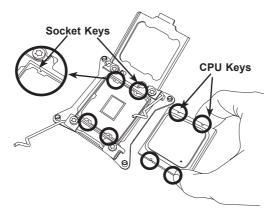
Once they are aligned, carefully lower the CPU straight down into the socket. (Do not drop the CPU on the socket. Do not move the CPU horizontally or vertically. Do not rub the CPU against the surface or against any pins of the socket to avoid damaging the CPU or the socket.)
