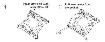
With the lever labeled 'Close 1st' fully retracted, gently push down on the lever labelled 'Open 1st' to open the load plate. Lift the load plate to open it completely.
