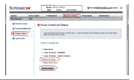
7. After the system powers on, the secondary boot block starts to initialize the essential hardware components and locates Super.ROM in the USB flash drive, which was mounted earlier. If Super.ROM is found, the on-duty boot block boots to it and finishes the rest of the POST processes. The system will automatically enter the BIOS recovery flash page in Setup at the end of POST. Move the cursor to **Proceed with flash update** and press **ENTER**.
